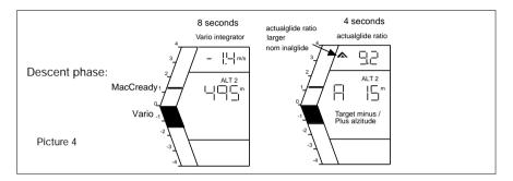
During the final approach, you must fly in such a way that the MacCready display in the analog display matches the last thermal integrator in the last thermal.
