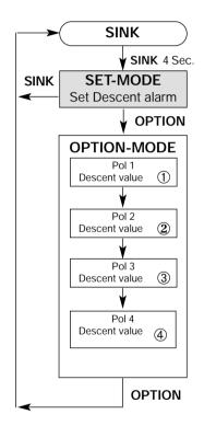
descent value. The value can be entered in steps of 0.1 m/s with the and keys. Pressing the key again increases the speed each time by 2 km/h up to 120 km/h.
