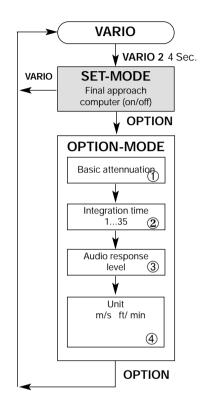
The audio response point can be adjusted at the third level. The audio response point can be adjusted from +2 cm/s to +40 cm/s. The current response point appears in the bar display and represents one tenth of the value displayed. E.g.: a display of 2 m/s corresponds to an audio response point of 20 cm/s.
